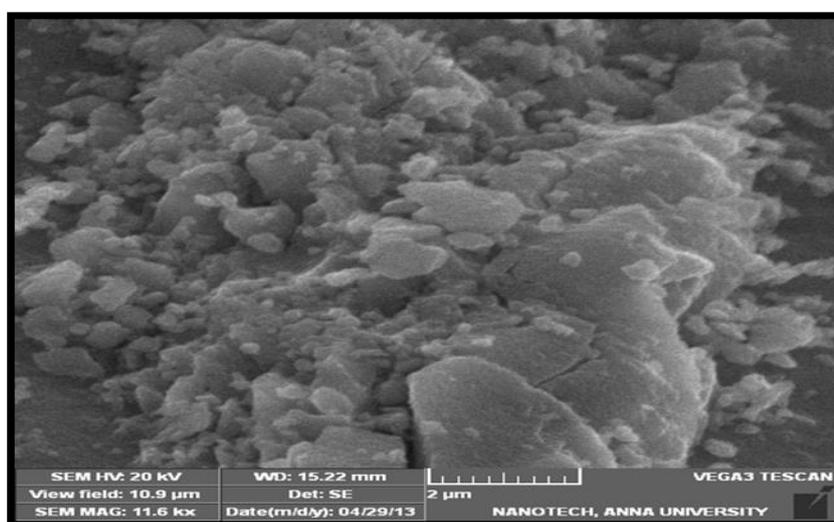
Figure.6 SEM Image of Titanium Dioxide Particles
