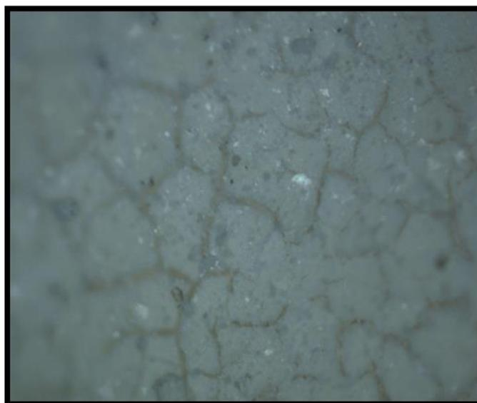
Figure. 5 Optical Microscope Image of Titanium dioxide Coated Clay Pellet Surface
